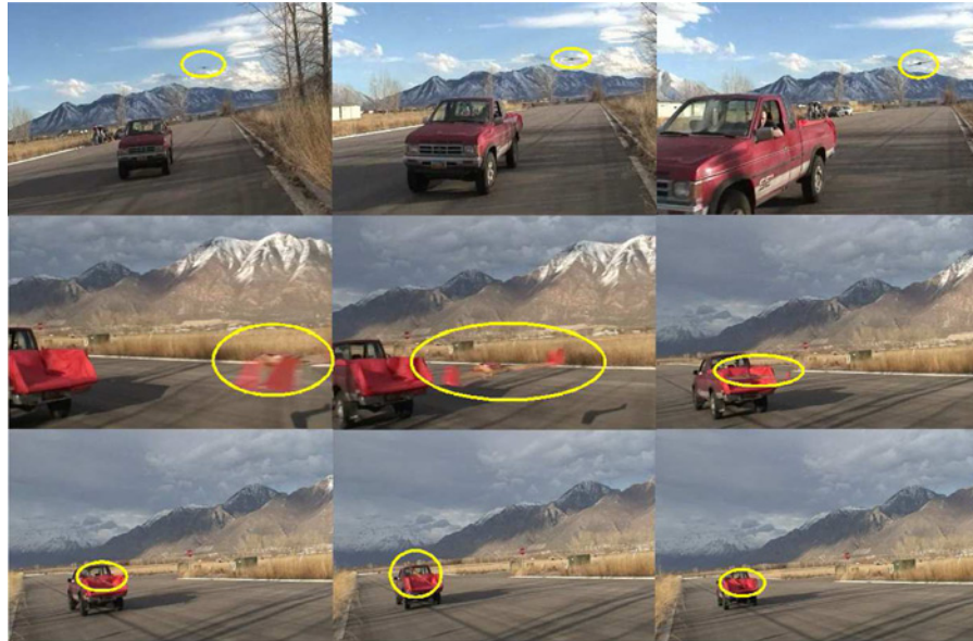
Fig. 16 Sequence of images showing successful landing on a moving platform.
